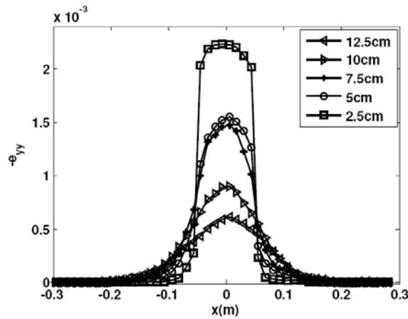
**Figure 13:** Vertical normal strain response for the packing that contains monodisperse mixture of particles.
