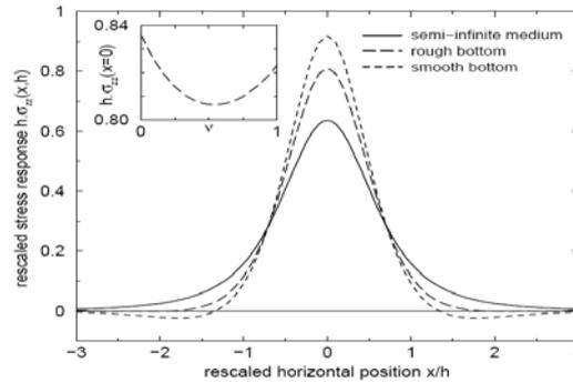
**Figure 12:** Experimental results of vertical normal stress response of rectangular assembly at the bottom layer for three different systems [9].
