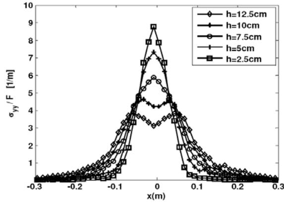
**Figure 4:** Vertical normal stress response at different depths of a system consisting of a bidisperse mixture of particles.
