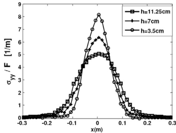
**Figure 10:** Vertical normal stress responses to a point source for a rectangular assembly of polydisperse granular material with a rough bottom.
