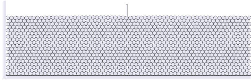
**Figure 1:** Rectangular packing of monodisperse particles on a smooth bottom with a load applied to a single grain at the top surface of the system.
