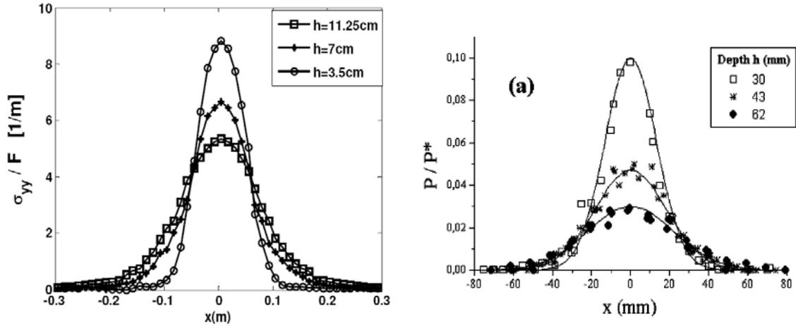
**Figure 9:** Vertical normal stress responses to a point source for a rectangular assembly of granular material with a smooth bottom, consisting of a polydisperse mixture of particles. The left-hand side of the figure shows simulation results, whereas on the right hand-side experimental results are displayed [11].
