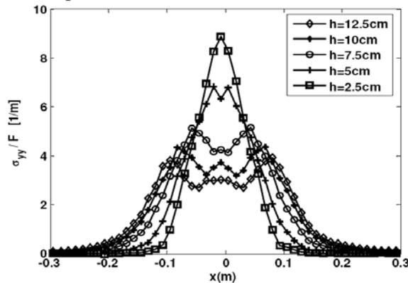
**Figure 3:** Vertical normal stress response at different depths of a system consisting of a monodisperse assembly of particles.
