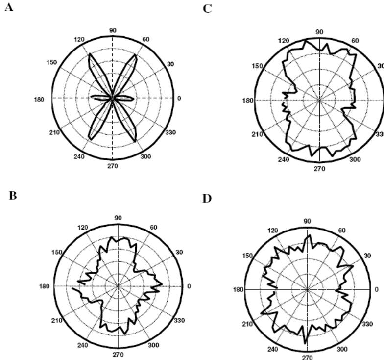
**Figure 2** Contact force angle distribution of the particles for the different packings. **A**, for monodisperse packing. **B**, for bidisperse packing. **C**, for pentagonal packing. **D**, for polydisperse packing.
