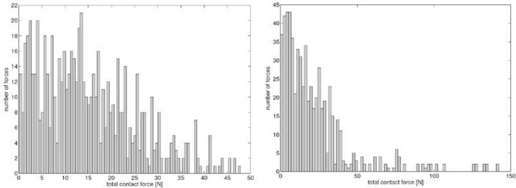
**Figure 8:** Left: force distribution in the monodisperse assembly with static friction coefficient  $\mu = 0.3$  for an external force  $F=100$  N. Right: the same for  $F=300$  N.
