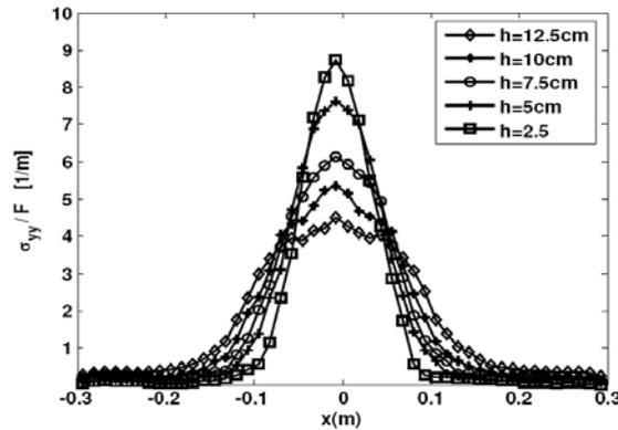
**Figure 5:** Vertical normal stress response at different depths of the system consisting of an assembly of pentagonal particles.
