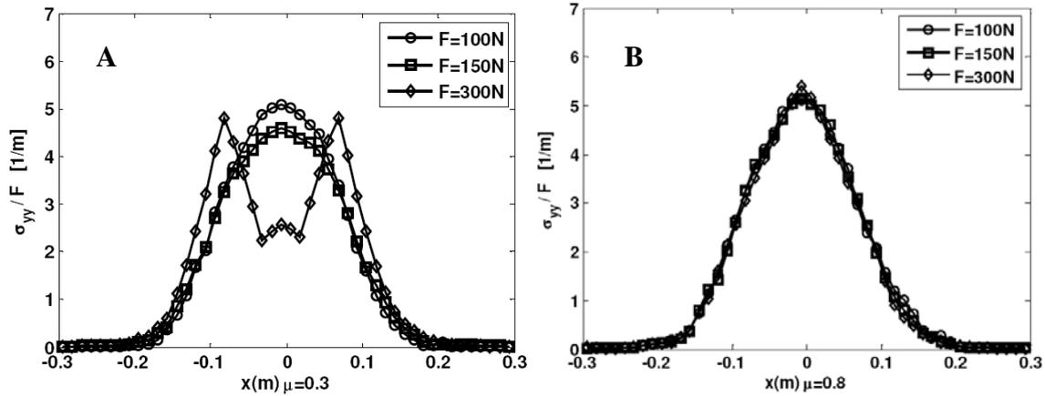
**Figure 7:** Vertical normal stress response for different values of applied loads at the bottom layer of the rectangular assembly. A: static friction coefficient  $\mu = 0.3$ , B: static friction coefficient  $\mu = 0.8$ .
