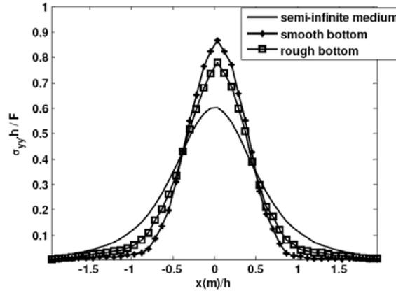
**Figure 11:** Simulation results for the vertical normal stress response of a rectangular assembly, at the bottom layer for two different systems, compared with an analytic solution.
