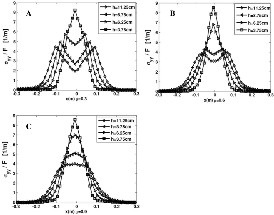
**Figure 6:** Simulation results of vertical normal stress response for different values of the friction coefficient. **A:**  $\mu = 0.3$ , **B:**, **C:**  $\mu = 0.9$ .
