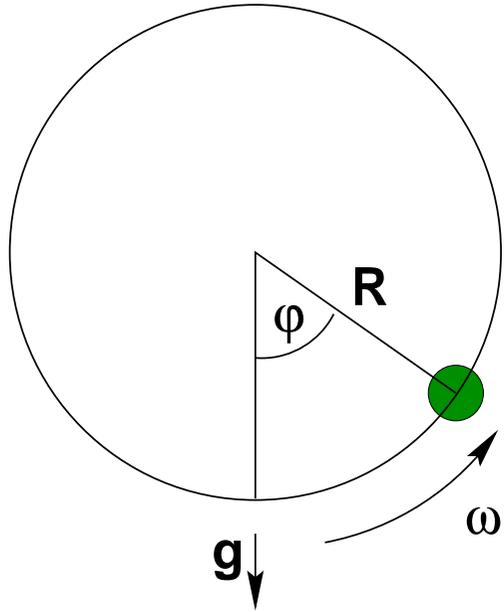
We want to investigate the motion of a particle in a rotating drum and are interested in steady orbits. Also we want to test different laws for the friction force.
